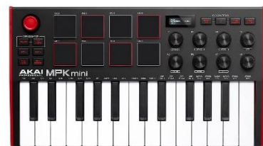
Figure 1: example of a lower to mid-range MIDI controller: AKAI MPK mini [2].
