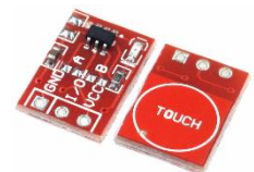
Figure 3: Capacitive Touch sensors for breadboarding [4].
